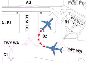
(Note: The lead-in lines are for aircraft nose-in guidance. For aircraft stands without dedicated pushback lines, ground crew may use the lead-in lines for pushback guidance. Diagram not to scale & for illustration only.)
